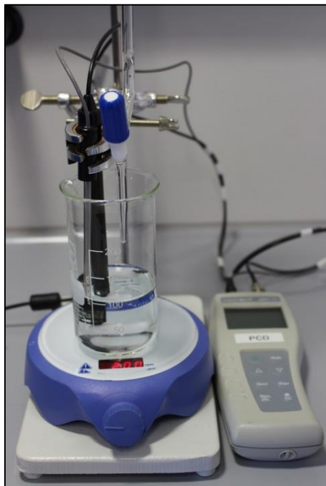
Figure 8 – Alkalinity Titration Apparatus
