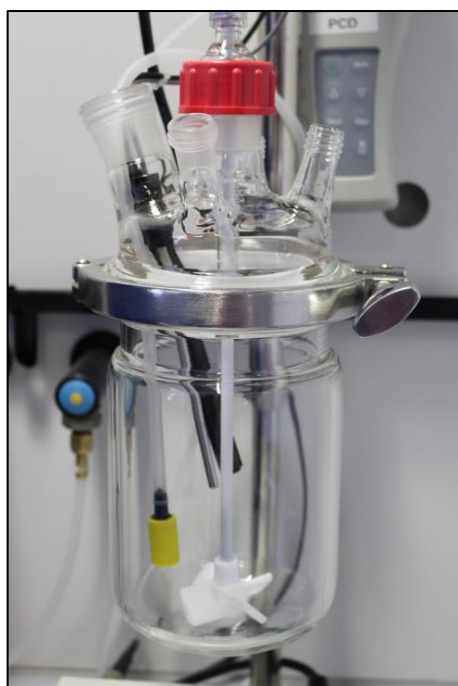
Figure 6 – 1 L Synthetic Water Batch (SWB) Apparatus
