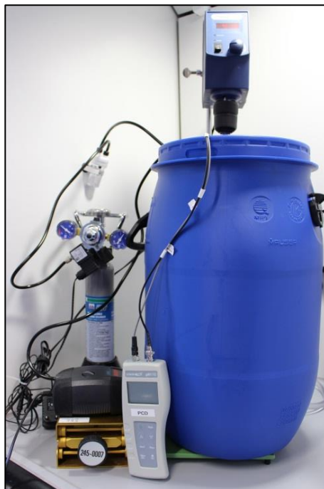
Figure 7 – Synthetic Water for Flotation (SWF) Apparatus
